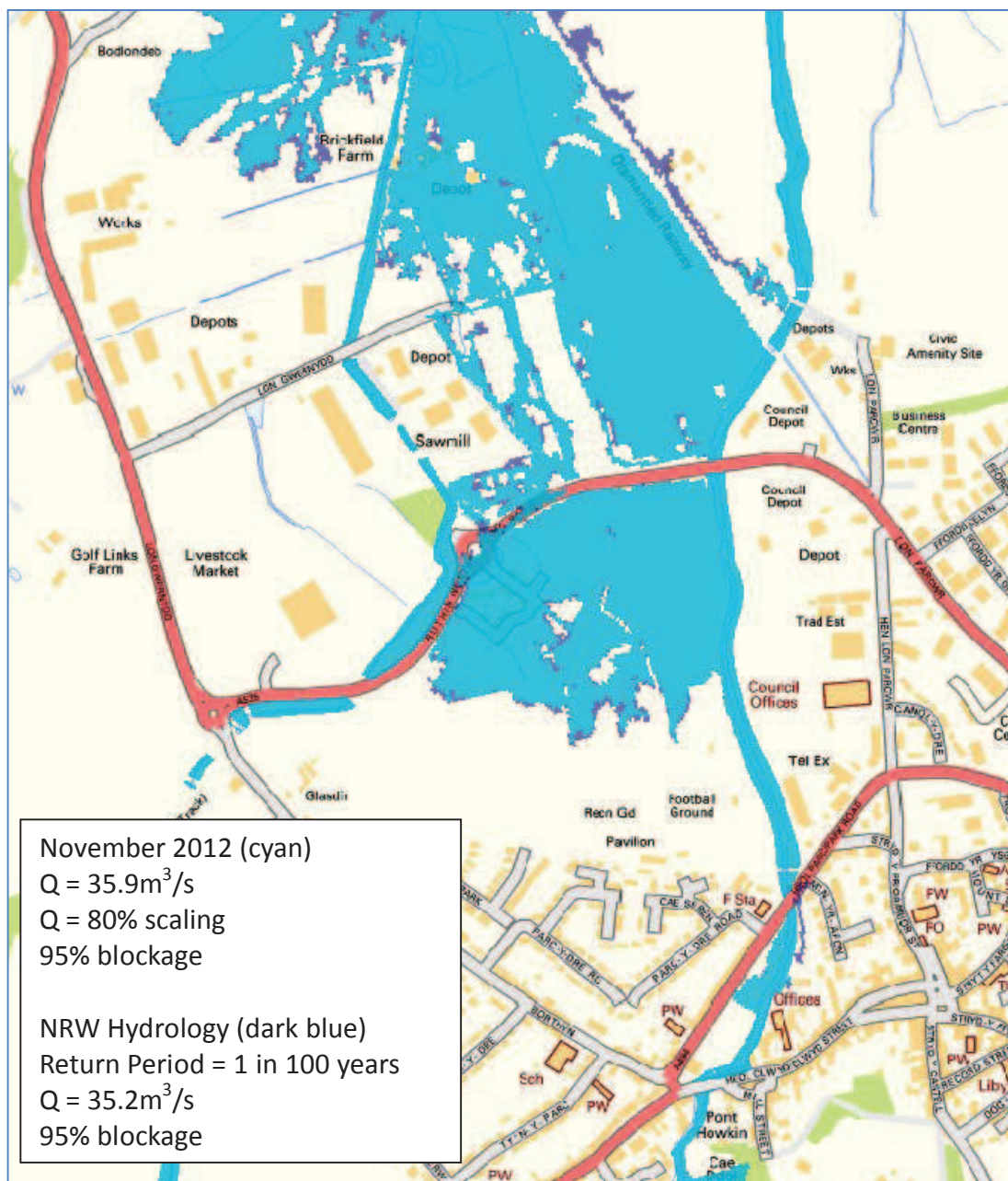
Figure 18 - Comparison of event hydrology scaled to 80% & NRW design hydrology Q100, both with 95% blockage
