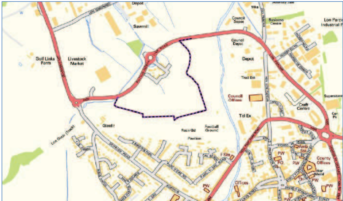
Figure 23 - Location of modelled Flood Defence around the Glasdir Estate. The line of the bund is for analytical purposes and does not indicate a suggested scheme.
