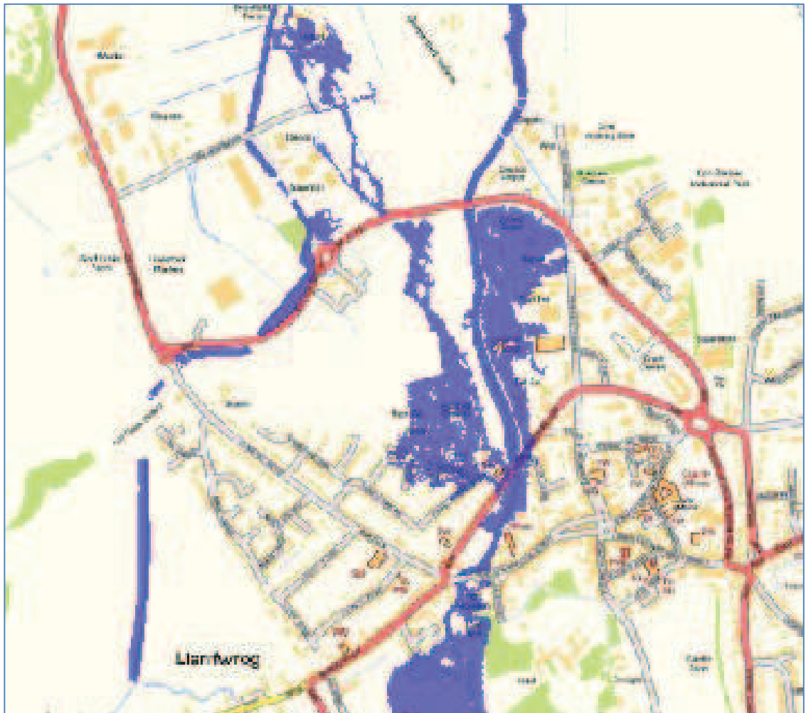
Figure 37 - Option 6 - ISIS TUFLOW Model Results for 1 in 100 year return period with Climate Change and 95% blockage
